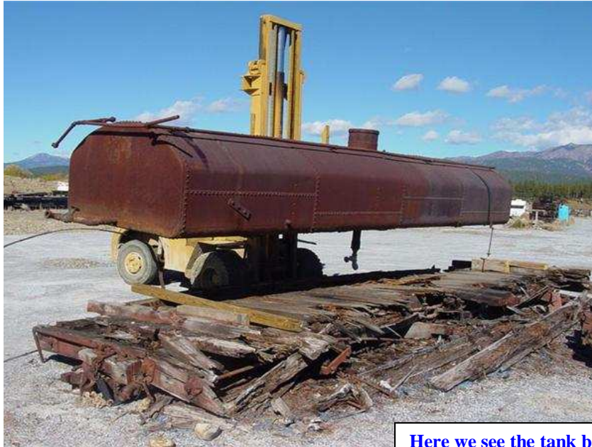
Here we see the tank being removed from the remains of the badly deteriorated car body.
